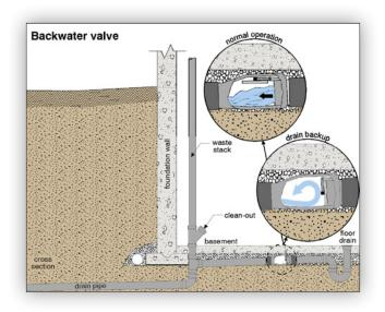
FLOOR Where there are separate sewers, the floor drains should go into the sanitary sewer **DRAINS AND** and gutters and downspouts should go into the storm sewer, or onto the ground several feet **DOWNSPOUTS** away from the building.
