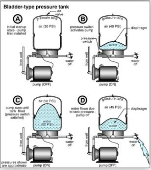
**WATERLOGGED** Over time, the air in the tank will be absorbed into the water and the tank will become 'waterlogged'. This means that the tank is full or nearly full of water. The pump will come on and off very quickly. This short cycling is hard on the pump, and air is added to the tank to correct the situation.
