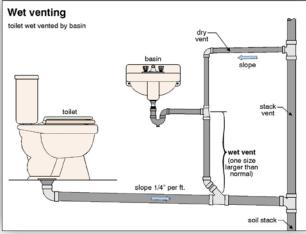
MATERIALS Vent piping may be cast iron, copper, galvanized steel or plastic. Because vent piping only carries air (no water) it tends to last a long time no matter what material is used.
