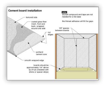
the tile and the tub is a weak spot. No matter what quality caulking is used, over a period of time, an opening will develop between the tub and tile. Although there is often a lip on the tub going up about one inch behind the tile, this does not always prevent water damage. Since bathtubs will flex to some degree, when filled with water and a person, this movement contributes to deterioration of the caulking.
