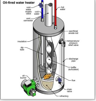
hot water, the heated water leaves the tank and cold water enters, triggering the thermostat and turning on the burner or element. If heated water flows out faster than the incoming cool water can be heated, we will run out of hot water. The larger the tank, the longer it takes to run out of hot water.
