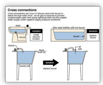
**BIDET IS** Some plumbing fixtures neces-ACCEPTABLE sarily create a situation which could lead to a cross connection. A bidet is a good example of this. A bidet has a water supply at the bottom of the bowl. This allows water to be directed up in a spray from the bottom center of the bowl. There is, of course, the potential for waste water in the bowl to get into this supply water. A special device (vacuum breaker) prevents water from flowing back into the supply plumbing.
