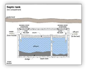
Most of the material entering the tank is in a liquid state. Within the tank, the majority of the solids are broken down to gases and/or liquids. The breakdown takes place as a result of bacterial action, both aerobic and anaerobic. The liquids are discharged from the tank into the tile bed. The gases escape through the plumbing vents in the home.
