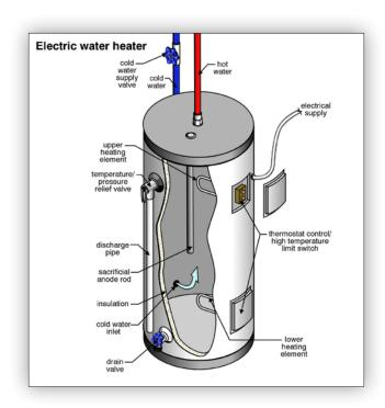
**RECOVERY RATE** When the hot water is depleted, the recovery rate becomes
