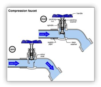
leaking washer will only allow water to drip into the fixture, while leaking packing will allow water to run onto a counter top, where it may cause damage.
