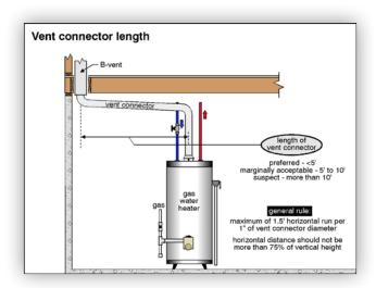
above the draft hood. Exhaust gases spilling out at the draft hood or burner may present a life-threatening situation. This problem requires immediate action. Some modern gas water heaters employ induced draft fans and high-temperature plastic venting that discharges out through the house wall. The vent materials were originally PVC, CPVC or ABS. In some areas these are replaced with special plastic vent pipes rated for the high exhaust gas temperatures.
