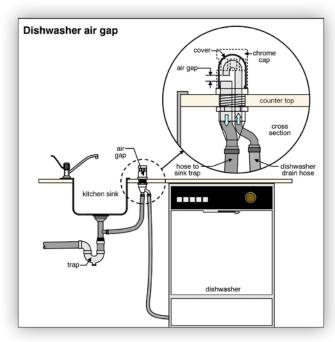
Air gap fittings are not required if the dishwasher has an integral backflow preventer.
