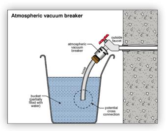
back through the hose into the drinking water. This may happen if the house water supply is shut off and partially drained for some reason, while the hose is in the pail. Back-flow preventers (like the atmospheric vacuum breaker in the illustration) on the hose bib can prevent this.
