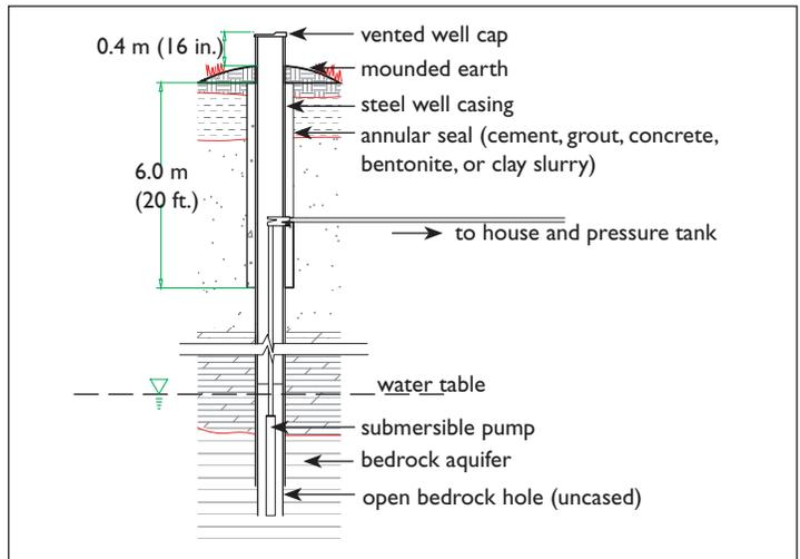
Figure 2 Drilled well
