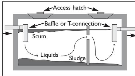
**Figure 4** Common septic tank
